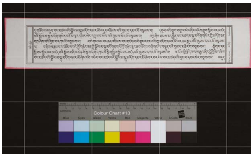
Figure 14. Electronic grids assist with the alignment of objects when copying. Photo © Patrick Sutherland, CC BY 4.0.
