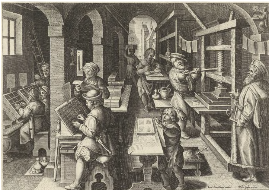
Fig. 1: Philip Galle, “Boekdrukkunst” (“Printing art”) (ca. 1589–1593), Rijksmuseum.org, http://hdl.handle.net/10934/RM0001.COLLECT.115331 . Printworks at the end of the sixteenth century, showing typesetting, the act of printing itself, and printed sheets hanging to dry.
